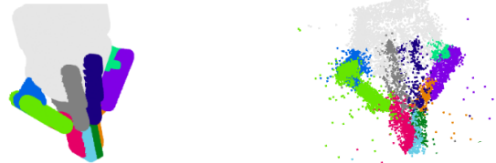
Fig. 4: We use a KNN-based classifier for segmenting links for articulated objects like parallel jaw grippers. We train a KNN model with the ground truth point labeling from the URDF model of the end effector.
